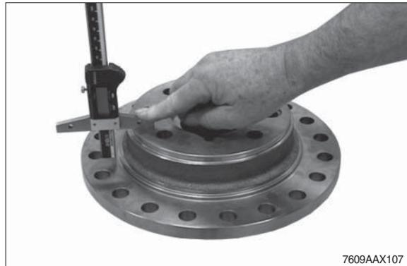
※ Any deviation from the required installation clearance is to be corrected with corresponding outer disks (s = 2.7, s = 2.9, s = 3.0, s = 3.1, s = 3.2, s = 3.3 or s = 3.5 mm), taking care that the difference in thickness between the left and the right disk package must only be 0.1 mm at maximum.
