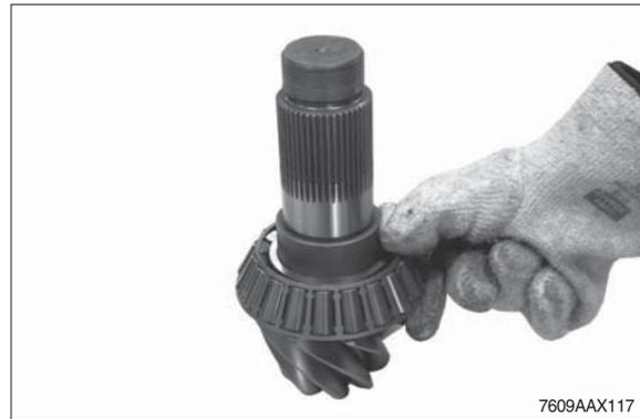
**Setting of rolling torque of input pinion bearing 0.15~0.41 kgf · m (1.11~2.95 lbf · ft) (without shaft seal)**
