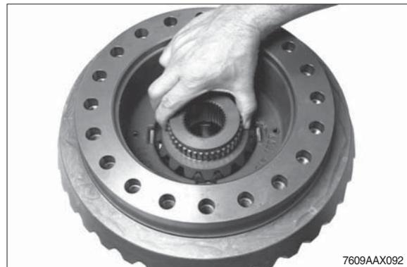
⑧ Fix the thrust washers into the housing cover by means of grease.
