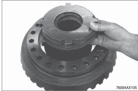
**Determine the installation clearance 0.2~0.7 mm**
