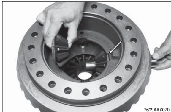
⑤ Insert spider gears with thrust washers into the differential housing and fix them with the two spider shafts (short).
