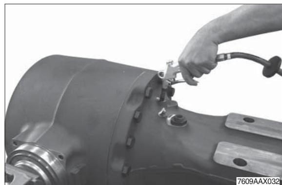
④ Heat slotted nut by means of hot air blower.
