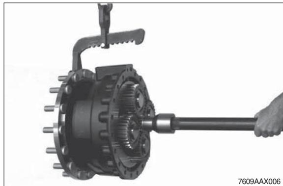
⑥ Fix output to assembly truck.
